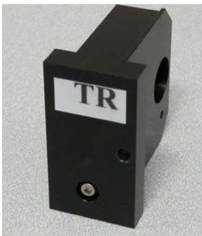
Figure 15: The “TR” cartridge, for time-resolved fluorescence assays
